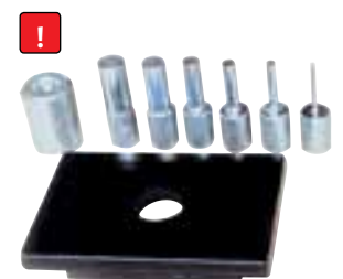
Placa furada com o conjunto de mandris, Ø 29, 24, 18, 14, 10, 5 mm
